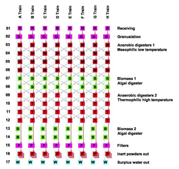
The envisaged plant will consist of a number of waste processing trains, columns A to H shown. Each train will consist of recieving modules (row 01).
